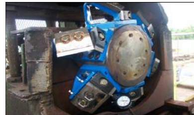
Simonds International A-C-T System installed in a 6 knife 5.5" End Dog Canter
